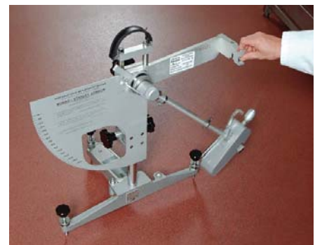
The Pendulum Slip Test can easily replicate the heel of a foot slipping on a floor and demonstrate the sustainability of safety flooring over many years
