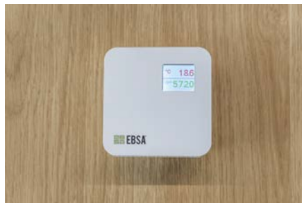
EBSA Control System for managing air quality in classrooms
