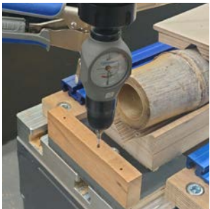
1 Calibrate robot arm to fixed real-life origin.
