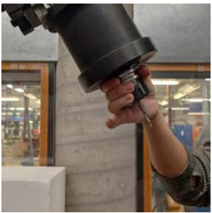
8 Fix drill head to robot arm.
