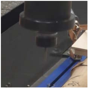
10 Make sure the drill bit spins before it reaches the cut piece and let it aircut one layer.
