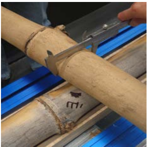
3 Measure the parameters for Grasshopper model input.
