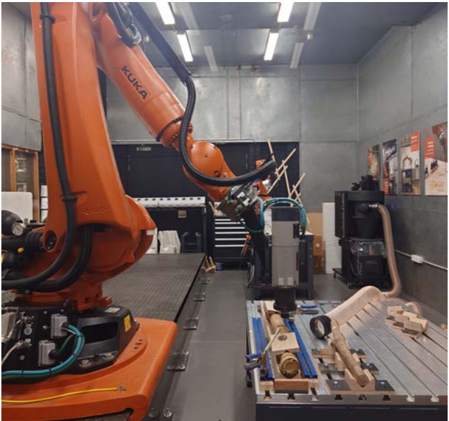
10 Make sure the drill bit spins before it reaches the cut piece and let it aircut one layer.
